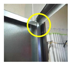
10. Position the top of the door in line with the top panel and insert M8 x 30 Cap Screw(16) DO NOT OVER TIGHTEN
