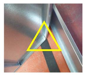
Position the bottom of the Door (2) onto the M8 x 25mm Stud (8).
