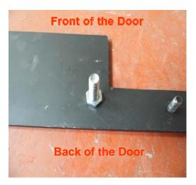
Fit the M8 x 25mm Stud (8) into the Door Base Plate (1) as shown for left hand hinge.
