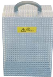
Type B Governor hood for Ø200 pulley, tall version; basically suitable for all standard controllers, f.e. SCHINDLER GBP(D), JUNGBLUT, etc. w=250, h=350, d=100-175 art. no. 78210 governor hood type B
