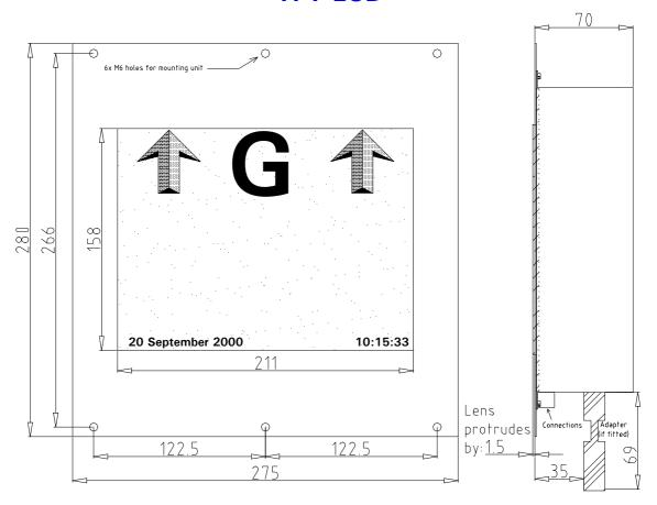
Faceplate Cut-Out: 164(h) x 217(w) mm Fixings: 6x M4x15mm studs
