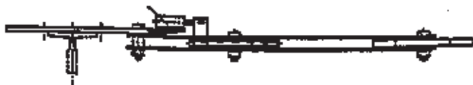
Fig. 3 Tension weight with counterweight (safety switch only in the plants in conformity to EN 81) type LK 200/250/300/315/200T with remote control
