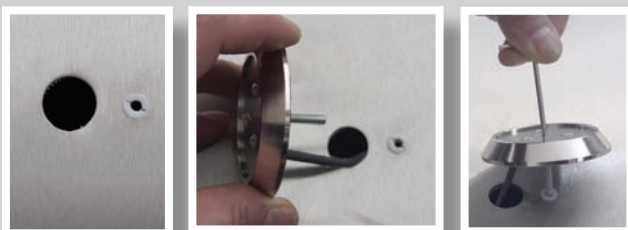
Example: Mounting with drill holes of 6.2mm for threaded bush and 12mm-30mm for the cable lead-through
