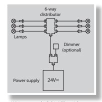
Wiring example CabinLED3 with max. 6 lamps and dimmer
