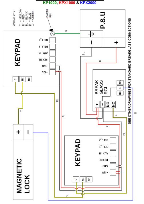
DOUBLE KEYPAD WIRING DIAGRAM
