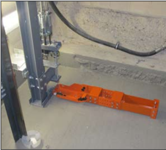
Example: Fixation of the maintenance support at the piston support
