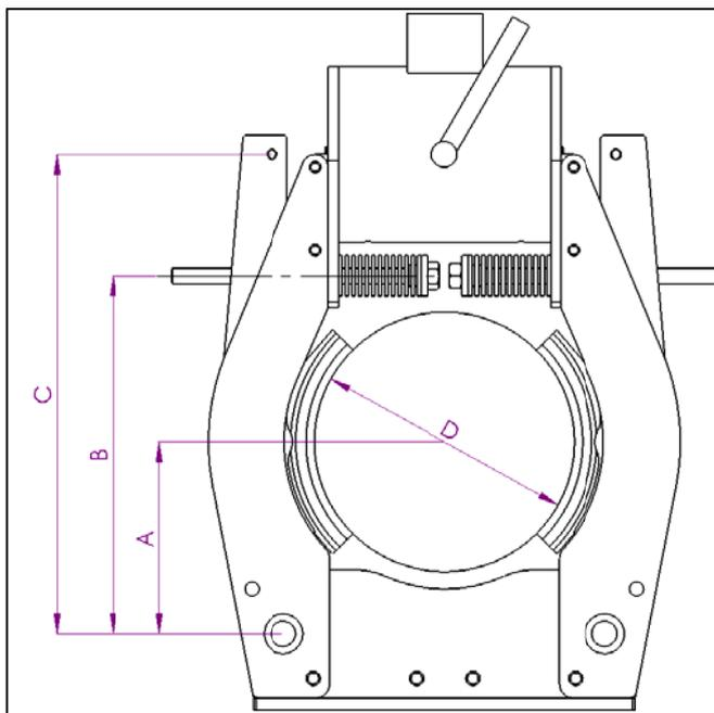
The braking moment is set by the spring preload. The spring preload of the spring has at least set so that the braking torque meets the requirements of the braking deceleration. When adjusting the spring preload, make sure that the preloaded spring force does not exceed the lifting capacity of the built-in magnets. (Pretension maximum)
