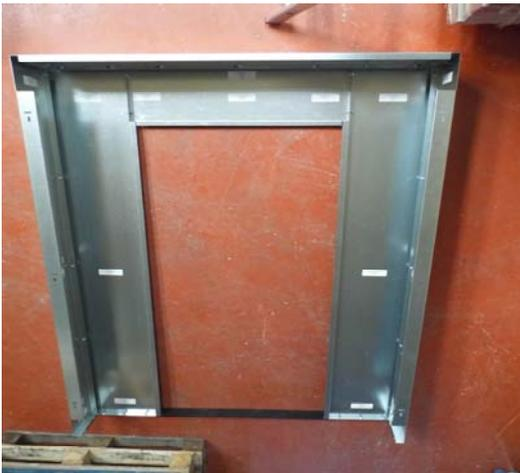
5. Connect the left (14), right (14) and top wall(13) panels to the three front panels (10),(11),(12)
