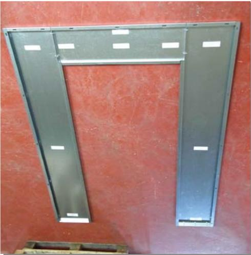
1. Connect the left (11) and right (10) hand side panel to the top panel (12).
