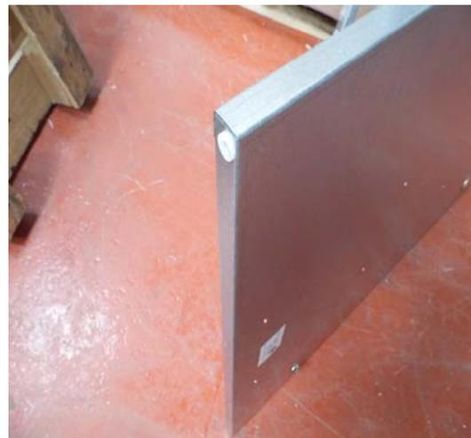
8. Insert the Nylon Bush (9) into the Door panel (2) at the top and bottom of the door.
