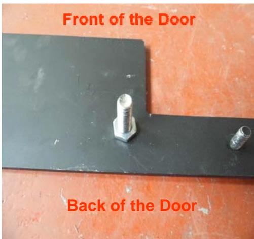
3. Fit the M8 x 25mm Stud (8) into the Door Base Plate (1) as shown for left hand hinge.
