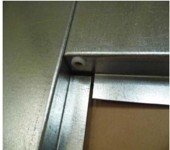
2. Insert the Nylon Bush (9) into the top left hand side of the top panel (12) as shown for left hand hinge.
