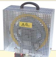
The cover consists of 8mm aluminium perforated sheet. Through this it is possible to make a sight check of the overspeed governor or of the shaft copying pulley at any time. With the provided butterfly nuts the hoods can quickly and easily be disassembled in case of inspections and maintenance.
