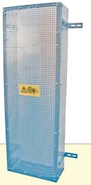
The diverter pulley cover is suitable for the protection of two pulleys on top of each other. This can often be found when the machine room is at the bottom. Through the 8mm perforated sheet it is possible to make a sight check of the running grooves without disassembling the cover. The cover can alternatively be attached to a concrete wall or to an iron frame. Both attachment variants are included in delivery.
