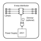
Please provide for a 12mm cable duct for the line connecting the 6 way distributor and the power supply unit at a suitable position in the cabin ceiling towards the cabin roof. Herefore use the enclosed rubber cable duct.
