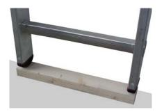
Put the ladder onto the provided mounting wood at the place where it should be mounted.There must be a distance of 60mm between the bottom of the ladder and the floor.
