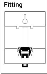
The EWS 102 can be mounted either on a DIN rail or on a flat surface using a single screw mounting aperture in the rear plate.
