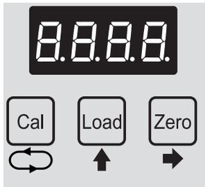
To begin the zero calibration, press the **Cal** and **Load** buttons together.
