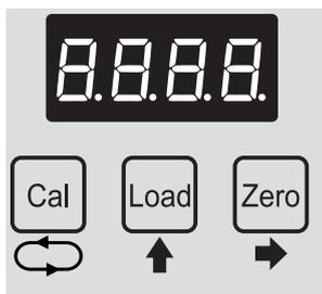
To begin the load calibration, press the **Cal** and **Load** buttons together.
