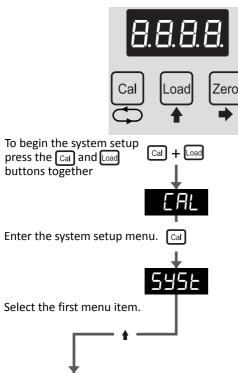
The system setup menu allows you to set and adjust various parameters
