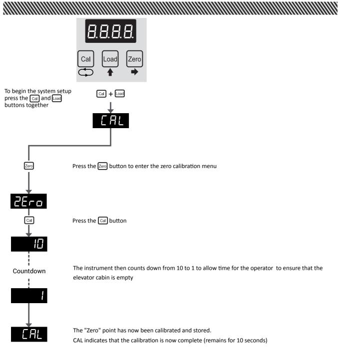
Press the Load button within 10 seconds to proceed to the Load Calibration
