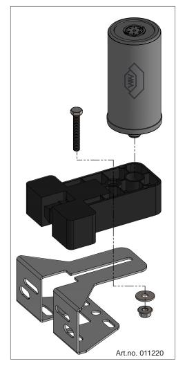
The brushes have to be adjusted centrally to the rail. The bristle on the front side shall be pushed in for about 3mm.
