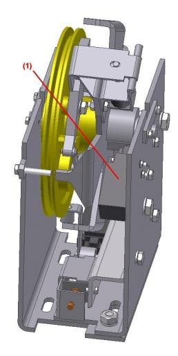
Therefore, the governors, whose rating speed is <u>1 m/s or lower</u>, will be provided with an overspeed switch that is triggered at the same time as the governor locks.
