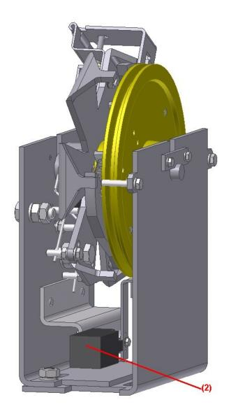
Remark: For installations in the well or similar, an automatic reset for this contact is possible. See afterwards
