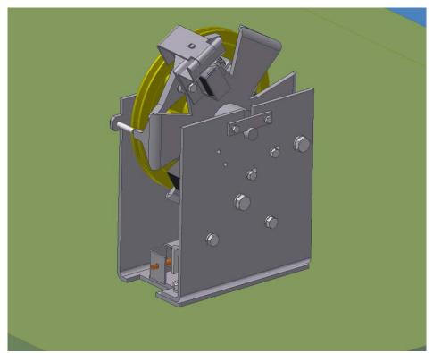
The ends of the rope (2) are attached to the linkage anchoring (1) thorugh eyes.
