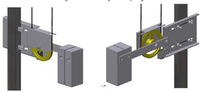
The rope must have enough tension (500 N on each side). In the event of tension loosening a rope slackening contact (1) connected to the installation security series will cut off the current.
