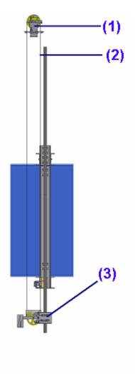
As it was indicated above, the governor is secured to the floor in the machine room or to the well.
