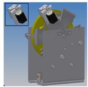
be released and, when there is no current, the mechanism will lock the governor. Therefore, it is advisable to use some sort of independent supply, so that, if there was a power cut in the installation and we have to move the car manually, this supply would be used to release the parking system and, at the same time, unlock the governor.
