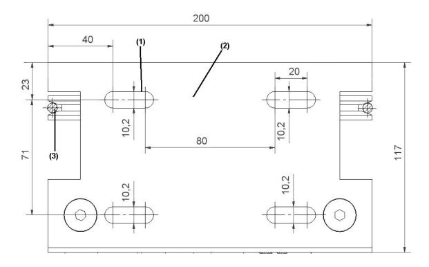
The above figure represents the bottom view of the governor base plate (2). The governor is anchored to the floor using the threaded holes (1) in the plate. The rope (3) and its position with respect to the base plate can also be seen in the drawing.
