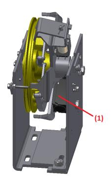
The governor has a built-in overspeed contact.
