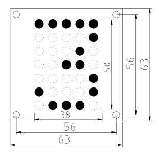
Faceplate Cut-Out: 60(h) x 48(w) mm Fixings: 4x M3x30mm Studs
