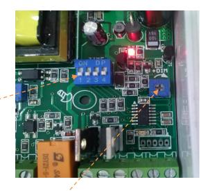
With the LED Spots connected, battery terminals connected and the power supply on, the LED spot lights will now operate – Red power light on. The emergency backup battery is now charging. The blue battery indication light will flash as per Battery Status Table.
