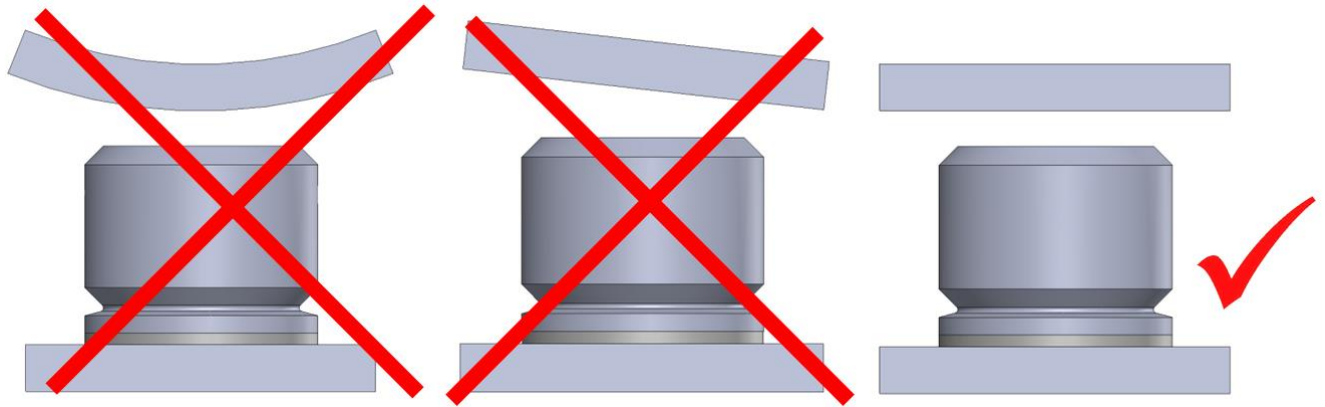
picture 4: even and parallel counter-pressure plates
